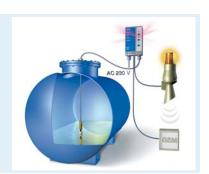
Application Designed to signal minimum or maximum levels of water, heating oil EL, L, M, oil/water mixtures and neutral, non-viscous and non-adhesive liquids in tanks. System owners are alerted when the supply runs low or if there is a hazard of overfilling.
