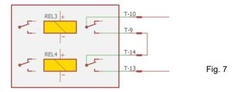
The signaling of the safety function with REL3 + REL4 is fixed in the device and cannot be changed. The relays are operated according to the closed-circuit principle, so that in the good state (safety function is not activated) the contacts on T-9/10 and T-13/14 are always closed.
