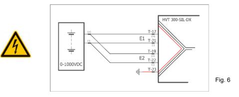
A line break monitoring is available for all 4 input lines, if the measurement signal has a value > 0 V. The transmitter then detects the line break and triggers the safety function. A series connection of the mA output with the REL3 or REL4 contact (NO) ensures that with the triggering of the safety function, the mA value is always 0 mA.
