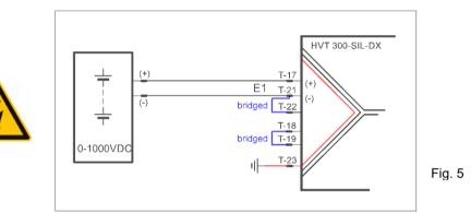
The absolute value measurement with only one measuring input is a possibility of interconnection with the signal source (e.g. 0-1000 VDC) and the transmitter, if the terminals T-18 and T-19 are bridged
