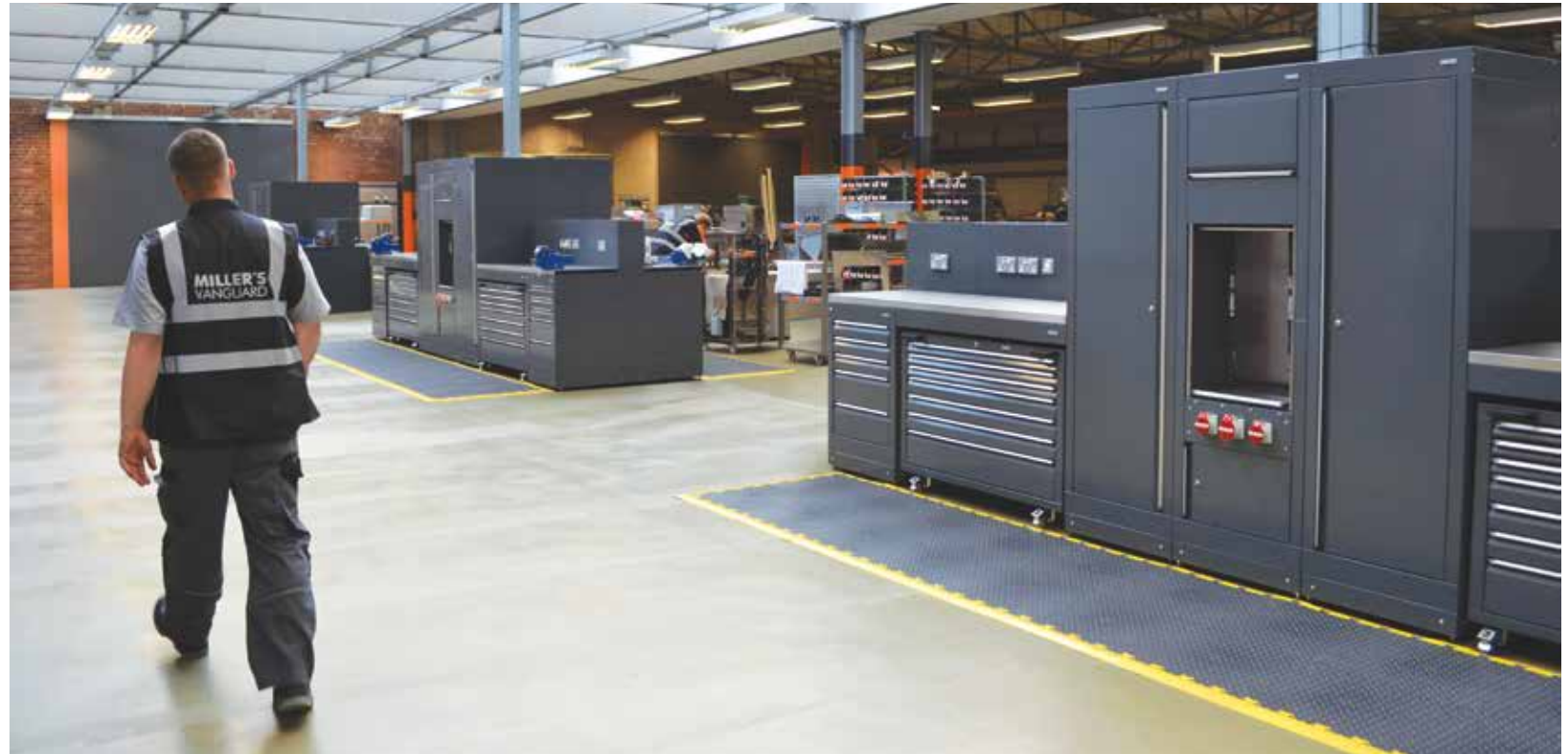
Main assembly workstations, with air and electrical management located centrally, allowing for an efficient work flow.
