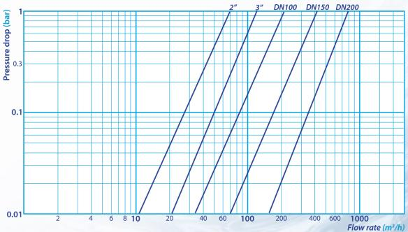
Head losses are referred to filters with 120 µm clean filtering mesh.
