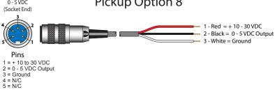
FIGURE 7 - WIRING FOR ACTIVE MAGNETIC PICK-UPS
