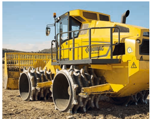
The service platform gives access to the maintenance area.
