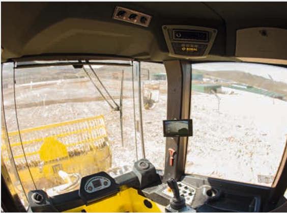
Cab with large windshields to ensure the best overview of the working environment.
