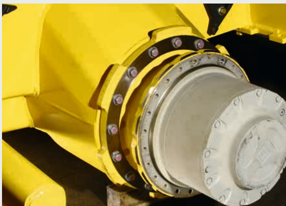
Two independent braking systems (hydrostatics used for service brake, multiple discs for the parking brake).
