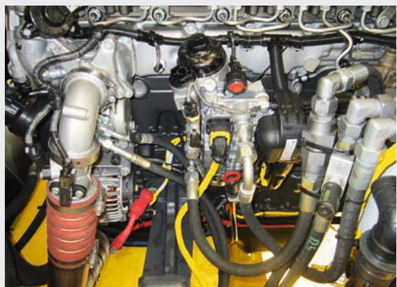
Multi-stage fuel filtering.
