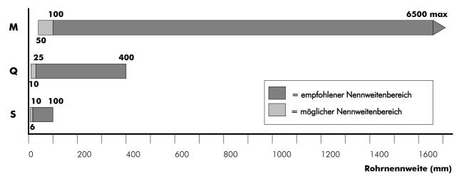
The **recommended diameter range** is the diameter range covered by a transducer under normal measuring conditions (signal damping mainly through fluid, no gas or solid in the fluid).
