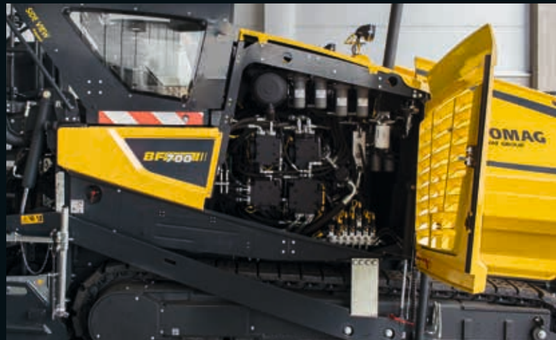
Generous: maintenance access.
