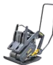
BP 20/50 Operating weight: 95 kg Centrifugal force: 20 kN Working width: 500 mm
