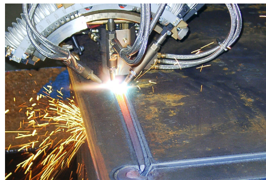
DAF/L cutting a K bevel.
