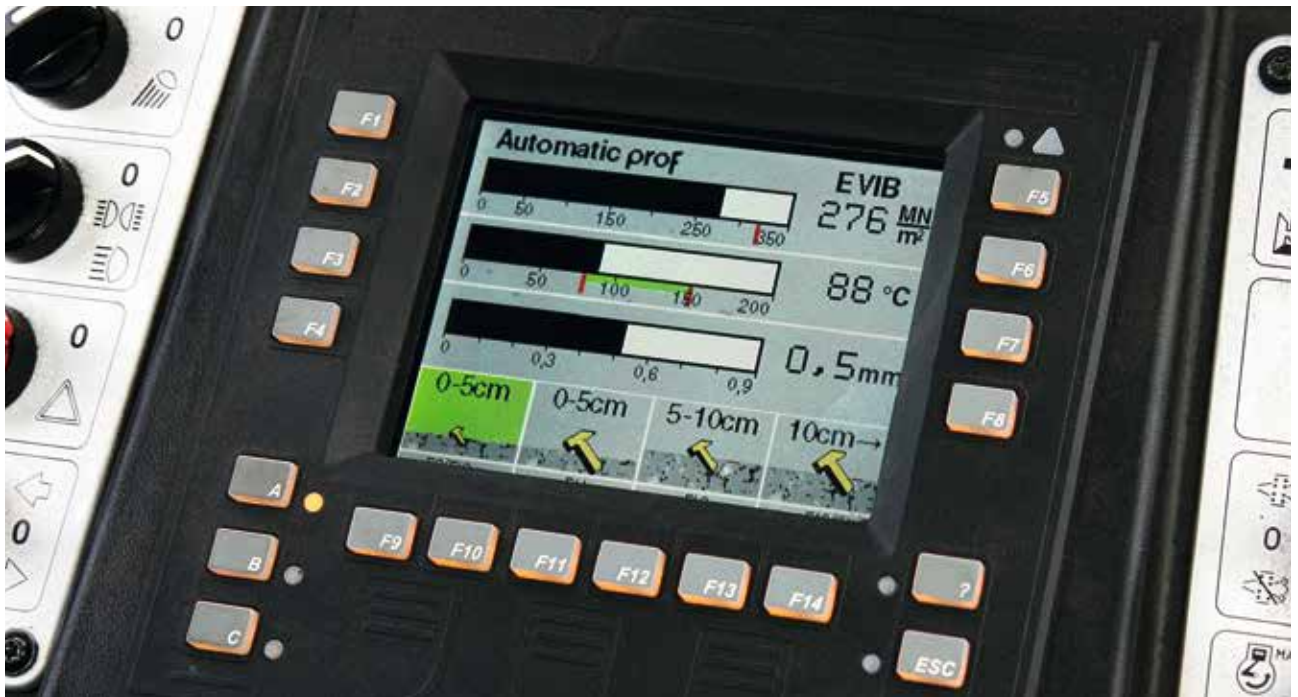
Clearly structured display: Always all values clearly in sight. Layer thickness pre-selection at a touch of a button.
