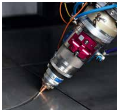
The infinitely rotating bevel head with magnetic collision protection enables bevel cuts up to 50°
