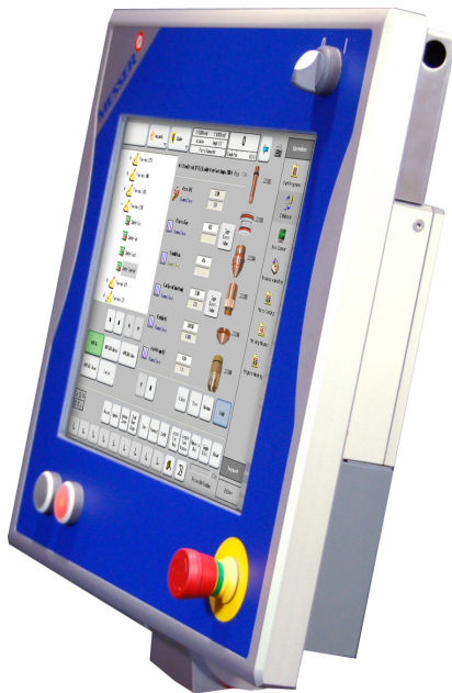
Hardened switches and industrial touchscreen.
