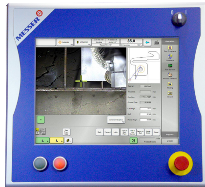
Video camera featured above (right) allows for fast, accurate plate alignment.
