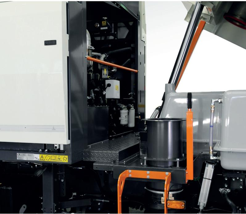
Safe and easy access to the auxiliary engine and filters via a large dedicated service platform.
