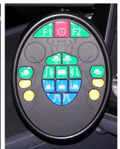
Scarab's CANbus control system has revolutionised the way sweepers are operated and maintained. Intuitive controls and a conveniently positioned colour monitor provide comprehensive levels of feedback to both operating and service personnel.
