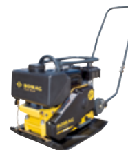
BVP 18/45 Operating weight: 91 kg Centrifugal force: 18 kN Working width: 450 mm
