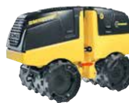
BMP 8500 Operating weight: 1,595 kg Centrifugal force: 72/36 kN Working width: 610 mm / 850 mm
