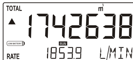
Fig. 4: Example of low-battery alarm.
