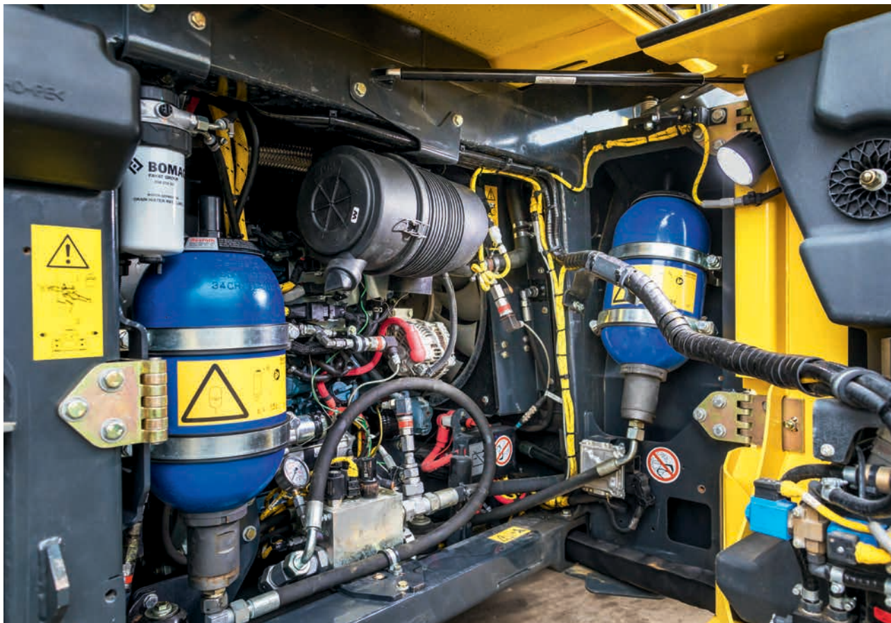
Highly efficient drive unit – diesel engine with hydraulic accumulator.
